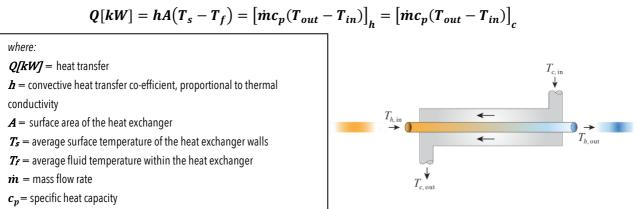
At a given rate of heat transfer (Q[kw]), the temperature of the fluid within the heat exchanger with Maxwell<sup>TM</sup> (**Tf**) will be closer to the temperature of the walls of the heat exchanger (**Ts**) demonstrating heat being exchanged more efficiently – a higher heat transfer coefficient (**h**).
